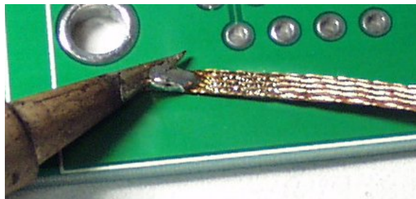
Figure 8.1: How to use a solder wick
