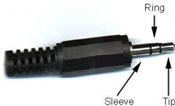
Figure 4.1: 3.5 mm stereo jack
