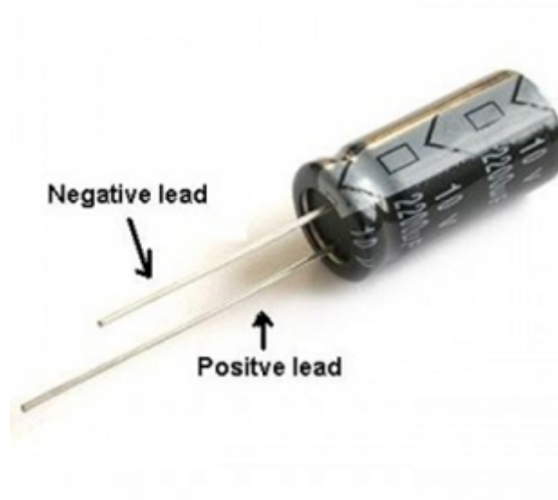
Figure 6.2: Elco pin layout
